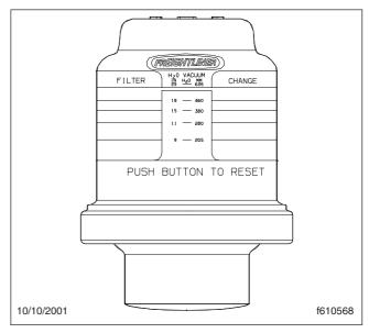
Fig. 3.13, Air Intake Restriction Indicator
