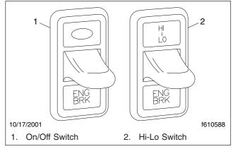
Fig. 13.4, Engine Brake Switches
