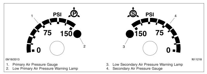
Fig. 19.8, Air Pressure Gauges
