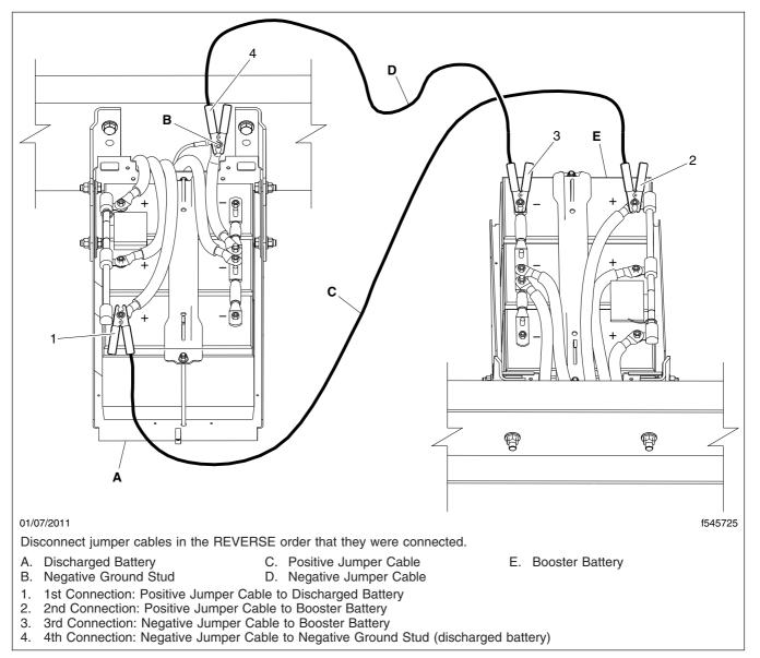
Fig. 17.3, Jumper Connections (three battery system shown for clarity)
