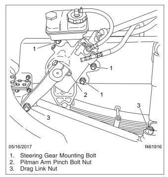
Fig. 15.14, Steering Gear Fasteners
