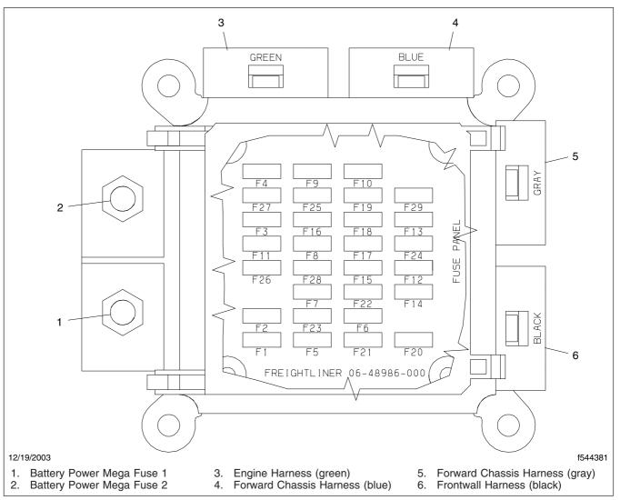
Fig. 6.2, Main PDM (top view)
