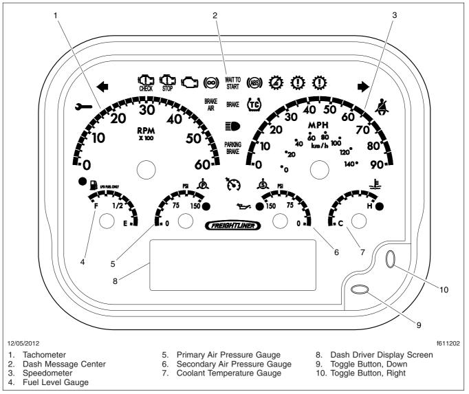
Fig. 19.11, Gauge Layout (typical, U.S.), LPG Engines
