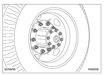
Fig. 15.8, Dirt and Rust Streaks from the Stud Holes
