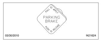
Fig. 4.17, Parking Brake Control Knob
