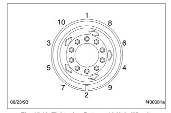
Fig. 15.10, Tightening Pattern, 10-Hole Wheels
