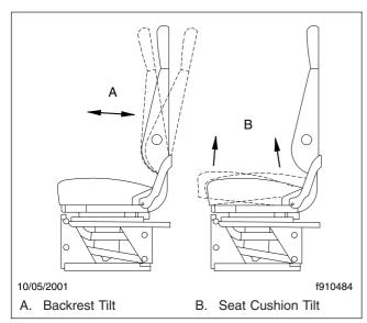
Fig. 5.8, Cushion Tilt Adjustments
