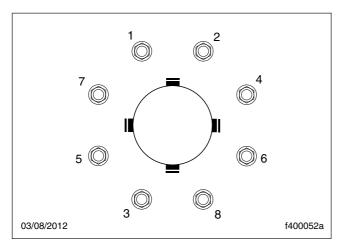
Fig. 15.11, Tightening Pattern, 8-Hole Wheels
