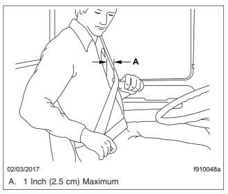
Fig. 5.18, Adjusting Shoulder Harness Clearance, Komfort Latch
