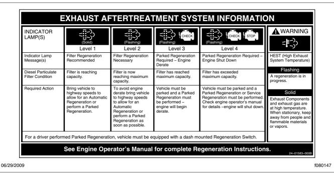
Fig. 9.3, Exhaust-Aftertreatment Warnings Reference Label
