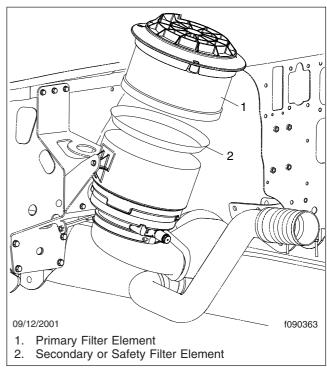
Fig. 15.2, Air Cleaner Filter Elements
