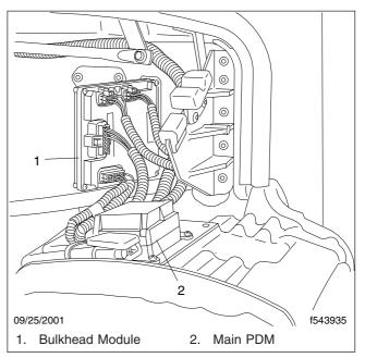
Fig. 6.1, Location of the Main PDM (under driver side hood, above fender)
