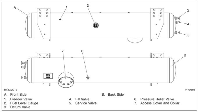
Fig. 19.4, Propane Tank System
