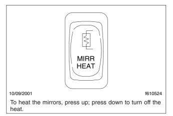
Fig. 5.3, Mirror Heat Switch
