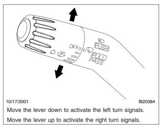
Fig. 4.6, Turn Signal Controls
