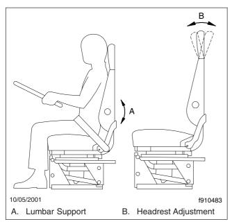
Fig. 5.7, Lumbar Support and Headrest Adjustment
