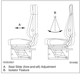
Fig. 5.6, Seat Slide Adjustment and Isolator Feature
