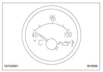
Fig. 3.17, Engine Oil Temperature Gauge
