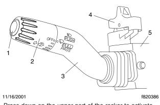
Press down on the upper part of the rocker to activate the hazard warning lights.
