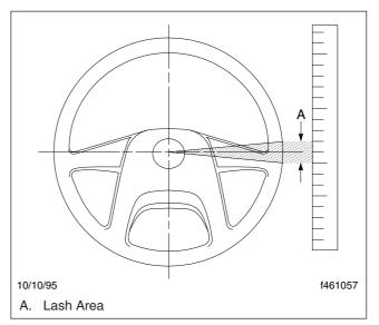
Fig. 15.17, Measuring Lash at the Steering Wheel
