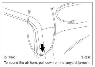
Fig. 4.11, Air Horn Control
