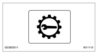
Fig. 3.6, Check Transmission Indicator
