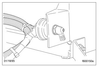
Fig. 2.2, Battery Disconnect Switch
