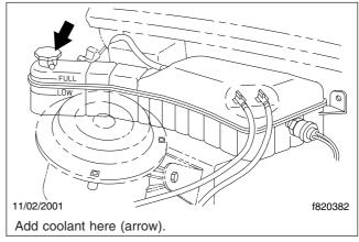
Fig. 15.1, Coolant Level Checking
