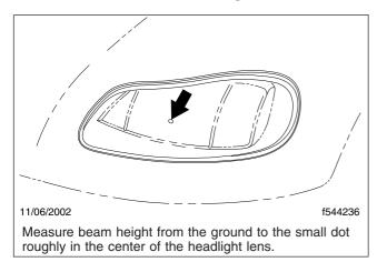
Fig. 18.1, Headlight Beam Height Adjusting Dot
