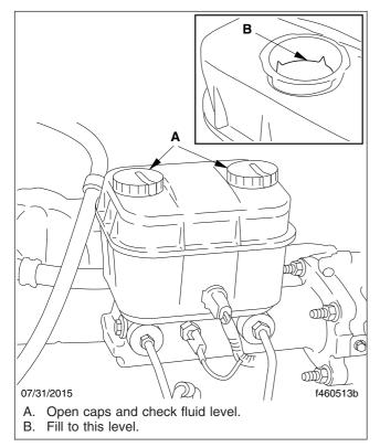
Fig. 15.16, Hydraulic Brake Reservoir
