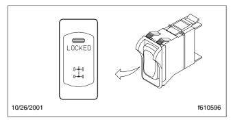
Fig. 11.1, Differential Lock Switch, Optional
