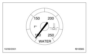
Fig. 3.9, Coolant Temperature Gauge
