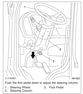
Fig. 12.2, Adjustable Steering Column
