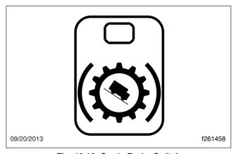
Fig. 19.10, Grade Brake Switch
