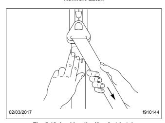
Fig. 5.19, Locking the Komfort Latch
