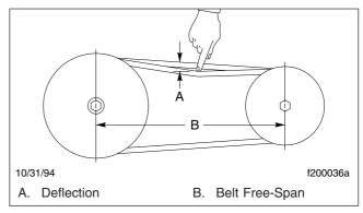
Fig. 15.15, Checking Belt Tension
