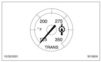
Fig. 3.18, Transmission Fluid Temperature Gauge
