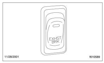
Fig. 13.3, Exhaust Brake Switch
