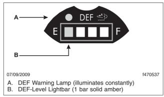
Fig. 9.8, DEF Level Low-Initial Warning
