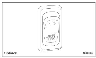
Fig. 4.19, Exhaust Brake Switch
