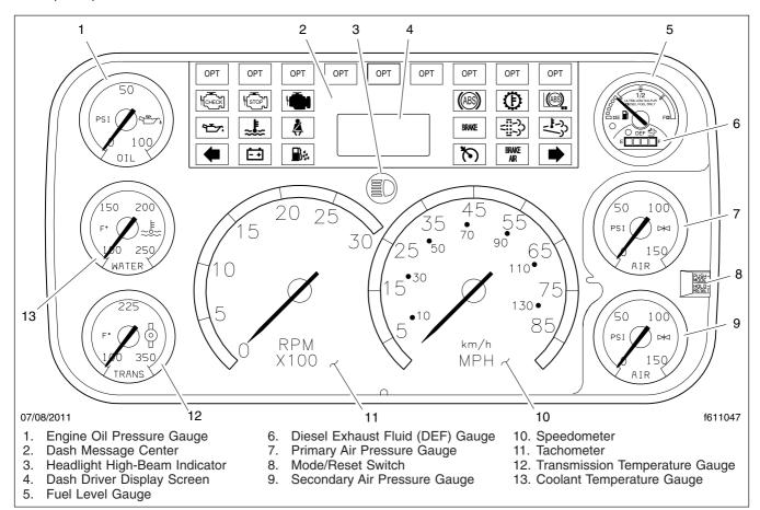
Fig. 3.1, Gauge Layout (typical, U.S.), EPA10 and Newer Engines
