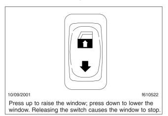
Fig. 5.1, Power Window Switch
