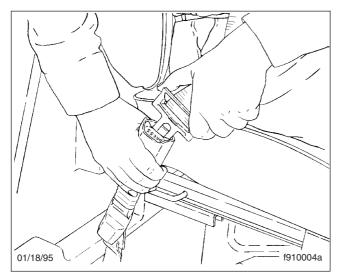
Fig. 5.17, Fastening the Three-Point Belt
