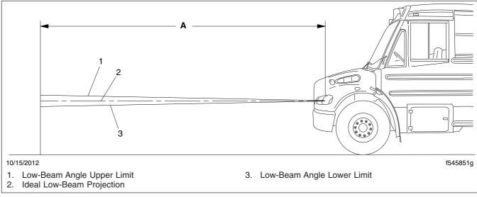
Fig. 18.3, Vertical Low-Beam Headlight Variation Limits
