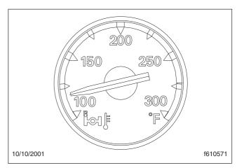
Fig. 3.15, Axle Oil Temperature Gauge
