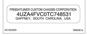
Fig. 1.2, Vehicle Identification Number, Typical
