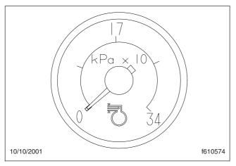
Fig. 3.19, Turbo Boost Pressure Gauge
