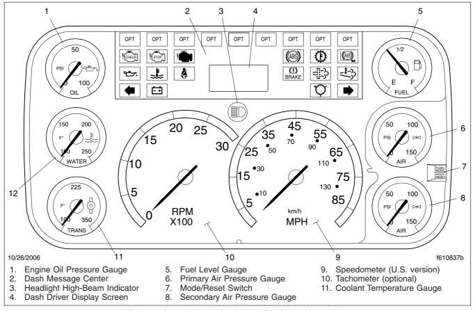
Fig. 3.2, Gauge Layout (typical, U.S.), EPA07-Compliant
