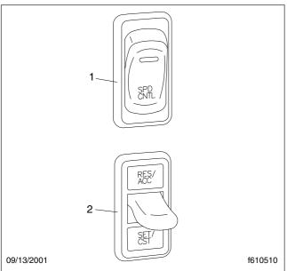
To turn the cruise control on, press the upper half of the On/Off (rocker) switch. To turn cruise control off, press the lower half of the On/Off (rocker) switch.
