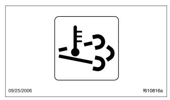
Fig. 9.2, High Exhaust System Temperature (HEST)
