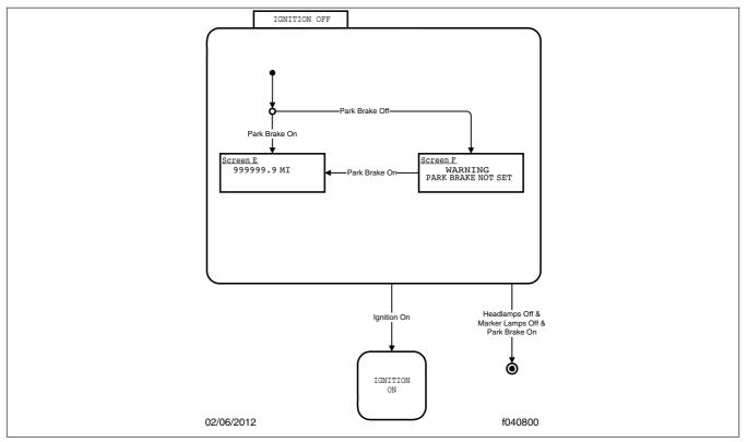
Fig. 19.24, Ignition Off (shown when ignition is keyed OFF)
