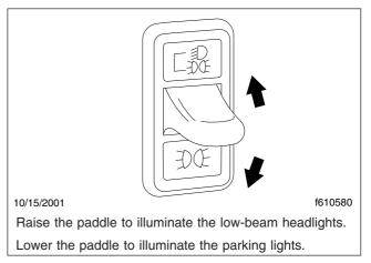
Fig. 4.2, Headlight/Parking Light Switch
