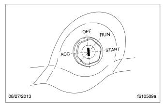
Fig. 19.1, Ignition Switch Positions
