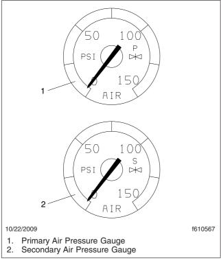
Fig. 3.12, Air Pressure Gauges
