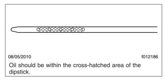
Fig. 15.5, Oil Dipstick (LPG engine)
