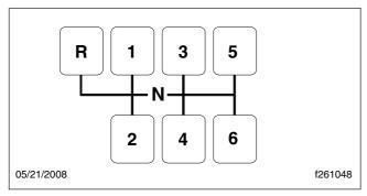
Fig. 10.4, Shift Pattern, 6-Speed FS and FSO Models
