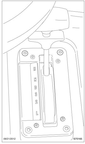
Fig. 10.1, T-Handle Shifter (standard)
