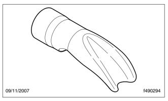
Fig. 9.12, Exhaust Diffuser
