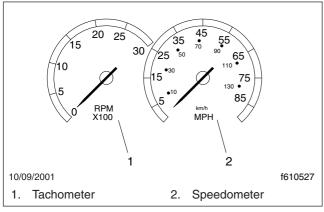
Fig. 3.7, Speedometer and Tachometer
