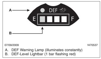
Fig. 9.9, DEF Level Low—Critical Warning
