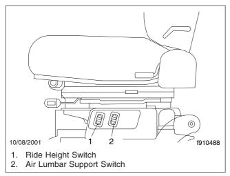
Fig. 5.14, Air Controls, Sears Seat
