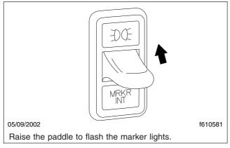
Fig. 4.4, Marker Light Interrupt Switch
