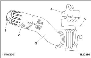
Press down on the upper part of the rocker switch to activate the hazard warning lights.
