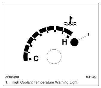
Fig. 19.9, Coolant Temperature Gauge
