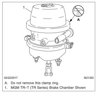
Fig. 15.12, Parking Brake Chamber Clamp
