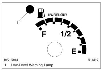
Fig. 19.7, Fuel Level Gauge
