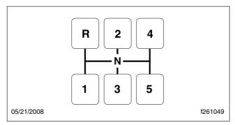
Fig. 10.3, Shift Pattern, 5-Speed FS Models
