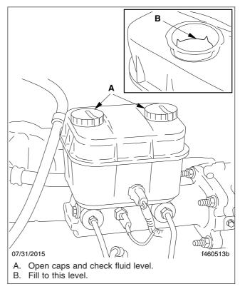
Fig. 13.2, Master Cylinder Reservoir
