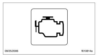
Fig. 9.14, Malfunction Indicator Lamp (MIL)
