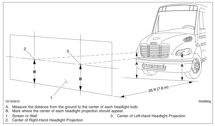
Fig. 18.2, Headlight Aiming Screen/Wall
