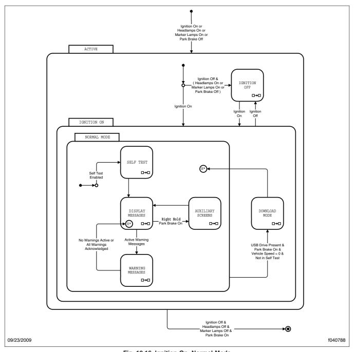
Fig. 19.16, Ignition On, Normal Mode
