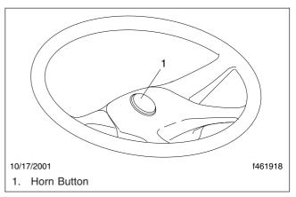
Fig. 4.10, Electric Horn Control
