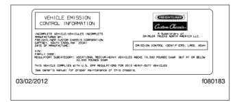
Fig. 1.5, Vehicle Emission Control Information Label
