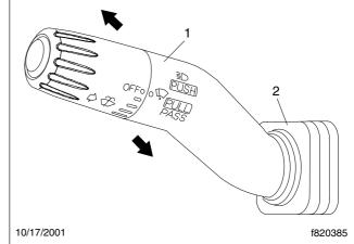
Move the lever forward to activate the high-beam headlights. Move the lever back to its original position to turn the high-beam headlights off.
