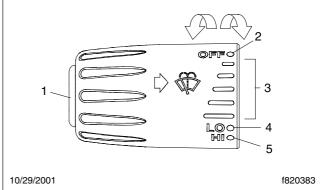
Rotate the control dial forward to turn the wipers on, or increase their speed.
